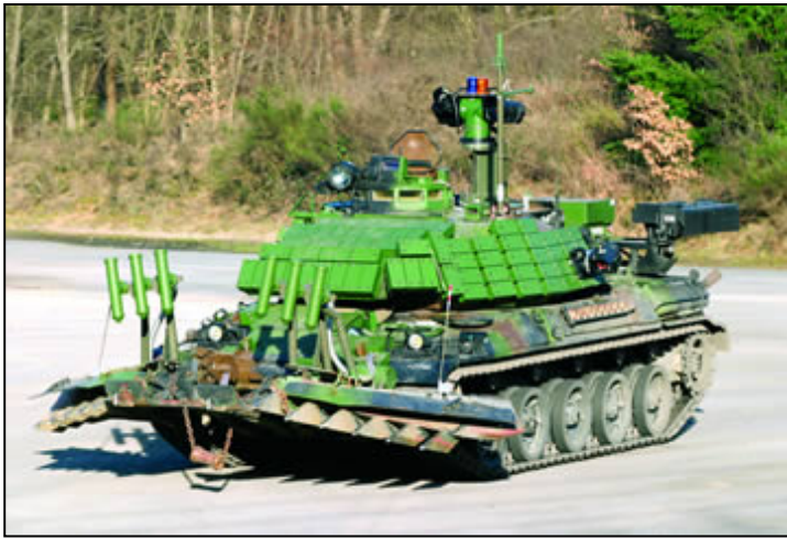
Giat's AMX30B2 remotely controlled tank is in service with the French Army for mine clearance operations. (Giat)
