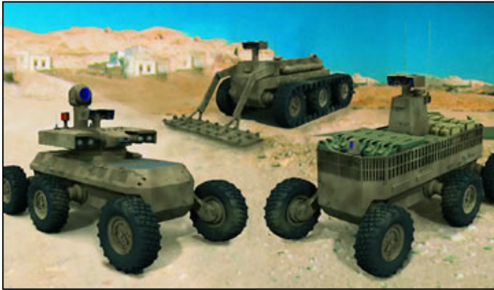
Lockheed Martin is developing a light assault (left), a countermine (centre) and a transport (right) variant of the Multifunction Utility/Logistics and Equipment (Mule) for the US Army's Future Combat Systems project. (Lockheed Martin)
