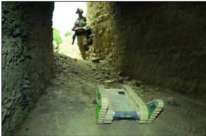
US forces are using iRobot's manpackable PackBot UGVs in Iraq and Afghanistan for reconnaissance and EOD missions. (US Army)
